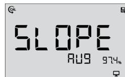
12. The average slope value is shown. The average slope is recommended to be between 92% to 102%.
