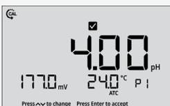
4. Once the reading is stable, press the **Enter** key.
