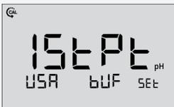
2. Rinse the pH/ATC electrode and place into the pH 4.01 buffer.
