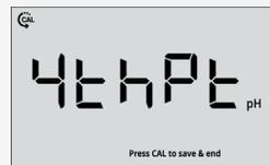
11. Press the **Cal** key to save and end the calibration. The **Cal** key can be pressed when either the "SAVED" or "4thPt" screens is shown.
