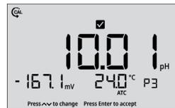
10. Once the reading is stable, press the **Enter** key.
