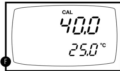
The meter will now compensate conductivity or TDS readings for the manually set temperature.
