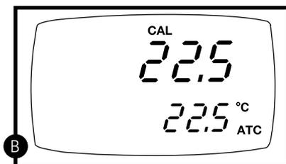
5. **Dip the cell into a solution of known temperature** (i.e. a temperature bath). Allow time for the built-in temperature sensor to stabilize.
