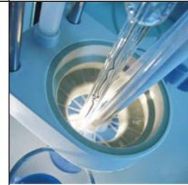
CoverUp™ lid handling device protects samples on the rack from contamination and prevents unpleasant odors.
