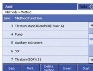
The T70 Excellence titrator controls two or more different titrations in a sample that run sequentially and fully automatically in series of up to 30 samples on the Rondo 30. The results are stored securely in the database of the LabX™ titration software.
