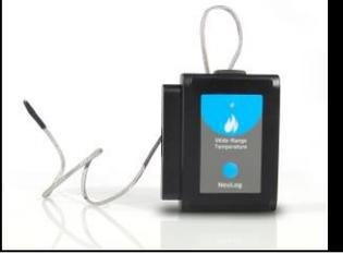
Because the metal wires have different properties both heat and electricity are conducted at different rates. Using the Seebeck Effect, a voltage is created in the wires. Different voltages are produced at different temperatures. The voltage is what is directly measured and then translated into a very accurate temperature reading.
