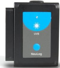
rays which strike the photodiode release free electrons which generate a voltage that can easily and accurately be measured. Voltage is converted into UVB density easily because they are directly proportional for the known surface area which is being measured.
