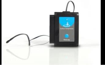
The surface temperature uses a partially exposed thermistor to rapidly detect temperature changes of surfaces compared to other thermometers which require the outer protective layer to change temperatures first. Temperature changes in the thermistor's wires act as variable resistance which is directly measured. When more heat is present the wires are slowed at a greater rate. The amount of resistance is rapidly measured and converted into a temperature readout almost instantaneously.
