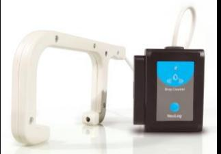
The NeuLog drop counter sensor uses an infrared beam which passes between the two endpoints of the sensor probe to determine drops. As liquid falls through the infrared beam infrared light is scattered and not detected at the infrared detector on the opposing side. Regardless of the liquids opacity or color, the infrared light will bend away from the detector. Every time there is a break in the infrared beam, a drop is counted at up to 100 samples per second.
