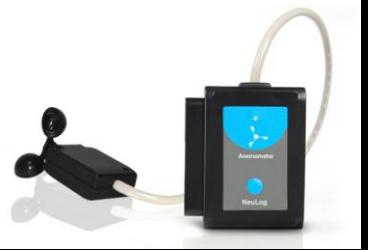
2. Connect the anemometer sensor to a USB-200 module (they directly plug together). Please note there is no calibration required for this sensor.
