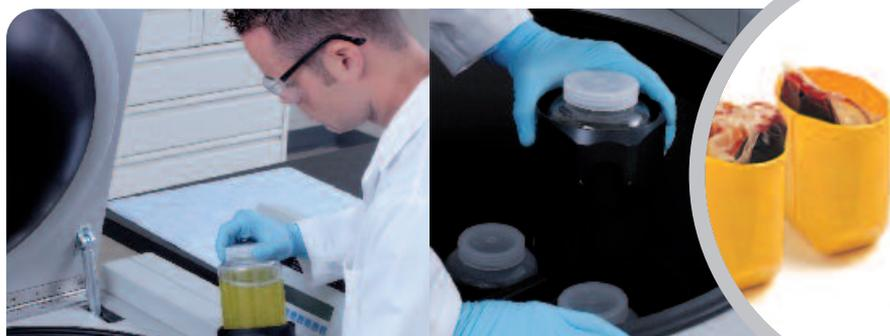
Buffy coat protocols can be optimized using the step-run mode, which automatically increments run speed in pre-programmed stages.
