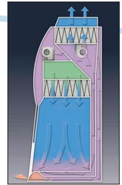
Side View: Airflow Diagram
