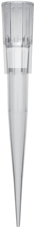
**FlexFit™** sealing technology makes an instant seal on the xPIPETTE. This patented feature consists of thick and thin ribs in the tip's seal area creating maximum flexibility. This flexibility allows it to easily conform to the shape of the pipette barrel and produce a secure seal.
