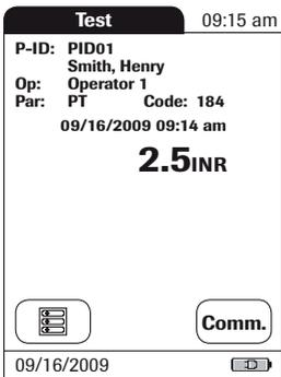
The result is displayed in the unit of measure you chose when setting up the meter. It is automatically saved to memory.
