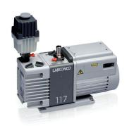
Rotary Vane Direct Drive Vacuum Pumps. These pumps are two-stage and oil-sealed with gas ballast control. Isolation valve seals the inlet to prevent oil and air contamination of the system in the event of power failure. Oil mist exhaust filter, vacuum pump oil and inlet adapters suitable for 1/2" OD and 3/4" OD are provided.
