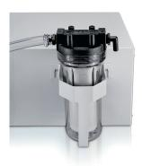
Chemical Trap. Traps are connected between the cold trap and the accessory vacuum pump to provide additional protection to the vacuum pump.
