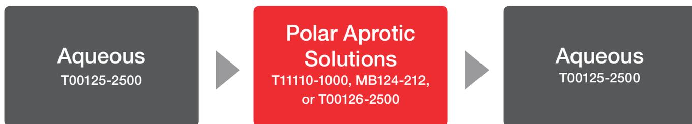
A thorough aqueous wash before and after using organic solvents can help to prevent the precipitation of proteins that can clog your instrument, cause sample contamination, and potentially cause premature replacement of your columns. Using the appropriate process will optimize peak shape, keep baselines smooth, and prevent precipitation.
