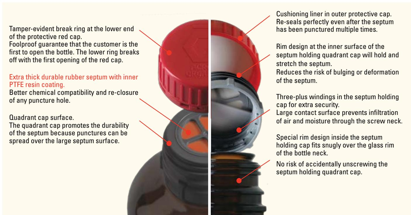
Tamper-evident break ring at the lower end of the protective red cap. Foolproof guarantee that the customer is the first to open the bottle. The lower ring breaks off with the first opening of the red cap.
