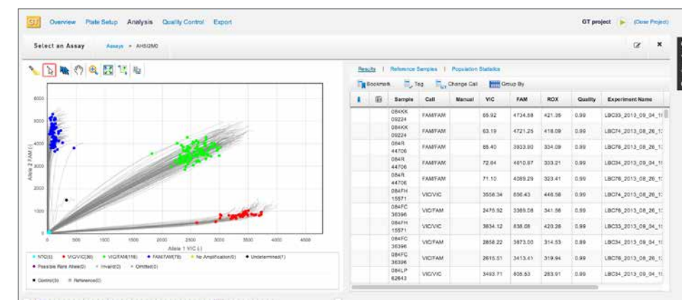
Figure 4. Genotyping analysis module. This module expands on existing TaqMan™ Genotyper™ software with improved visuals and integrated traces of allelic discrimination plots. The module allows for thorough quality control of SNP assays to accurately reflect true signals vs. background noise.
