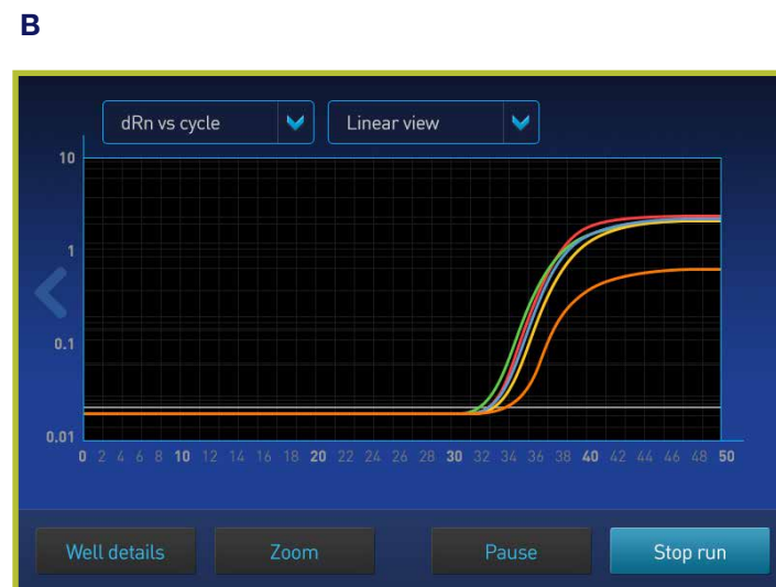
Figure 1. Graphical interface allows (A) easy editing of thermal cycling conditions and viewing of plate layout, as well as (B) viewing of amplification plots and drilling down to a subset of sample wells.
