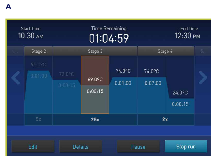
Figure 1. Graphical interface allows (A) easy editing of thermal cycling conditions and viewing of plate layout, as well as (B) viewing of amplification plots and drilling down to a subset of sample wells.
