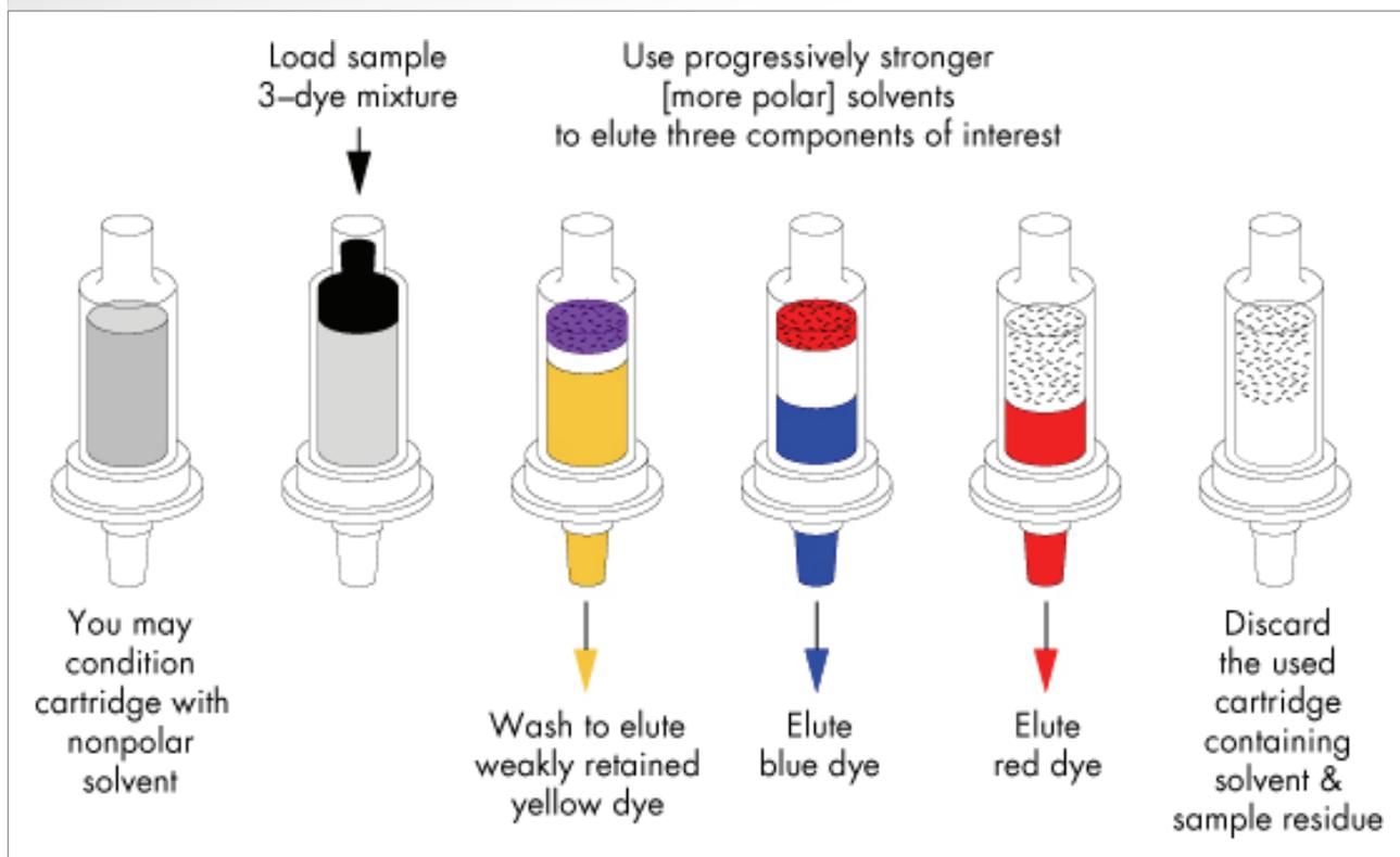
Kinetics are an important factor in SPE. The packed beds use larger particles than HPLC, meaning the rate of mass transfer is much slower. Driving the solution through the bed too quickly will result in some analyte passing completely through before it can be captured by the stationary phase. Sometimes, the difference between high and low reproducibility comes down to the strength of the vacuum system used to pull samples through the SPE cartridges.
