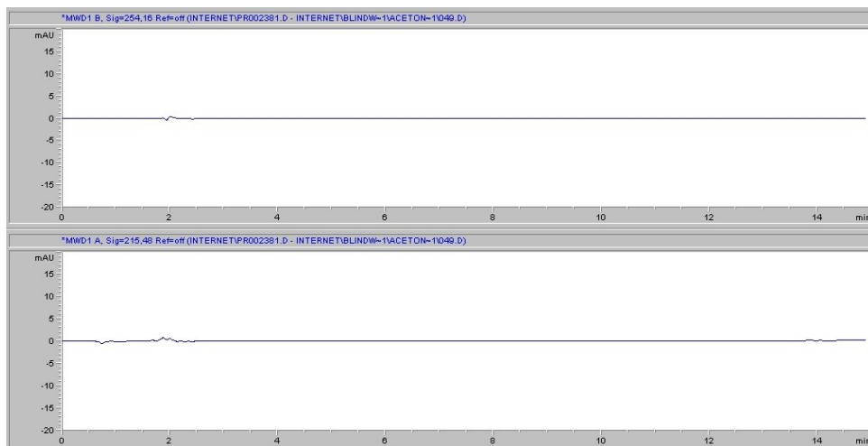
Fig 1. Representative chromatograms of solvents filtered through SPARTAN syringe filters and subjected to HPLC analysis. Top panel in each set of chromatograms shows results at 254 nm; bottom panel shows results at 215 nm.
