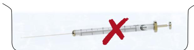
Do not immerse the entire syringe in solvent as this may damage the adhesive used to bond parts of the syringe. Clean externally by wiping with a tissue.
