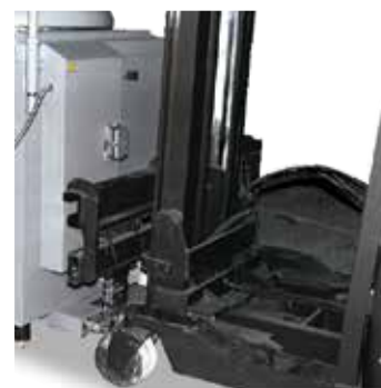
Slots under the furnace for the forklift forks
