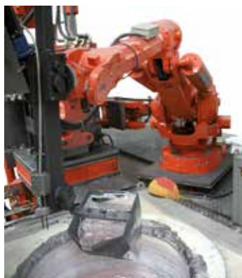
Bale-out of T 650/10 with robot
