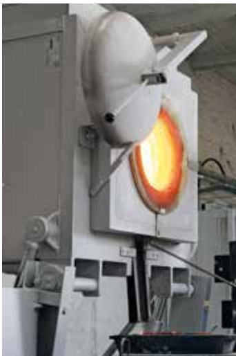
Tilting furnace K 40/13 with extended spout (sculpture foundry Knaak)
