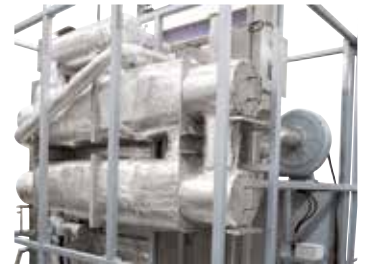
Counterflow heat exchanger for the forced convection chamber furnace N 2560/26 ACLS
