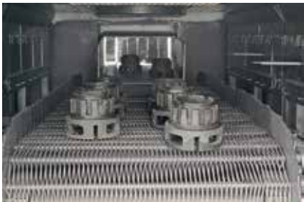
Mesh belt drive in a continuous furnace
