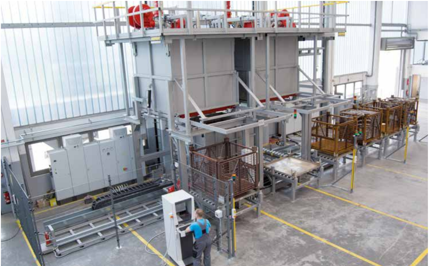
Fully automatic drop-bottom furnace plant, consisting of two drop-bottom furnaces, movable water bath and several loading and unloading positions
