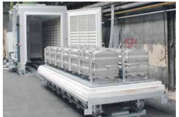
Bogie hearth furnace with gas supply system
