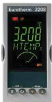
Eurotherm 3208 furnace controller
