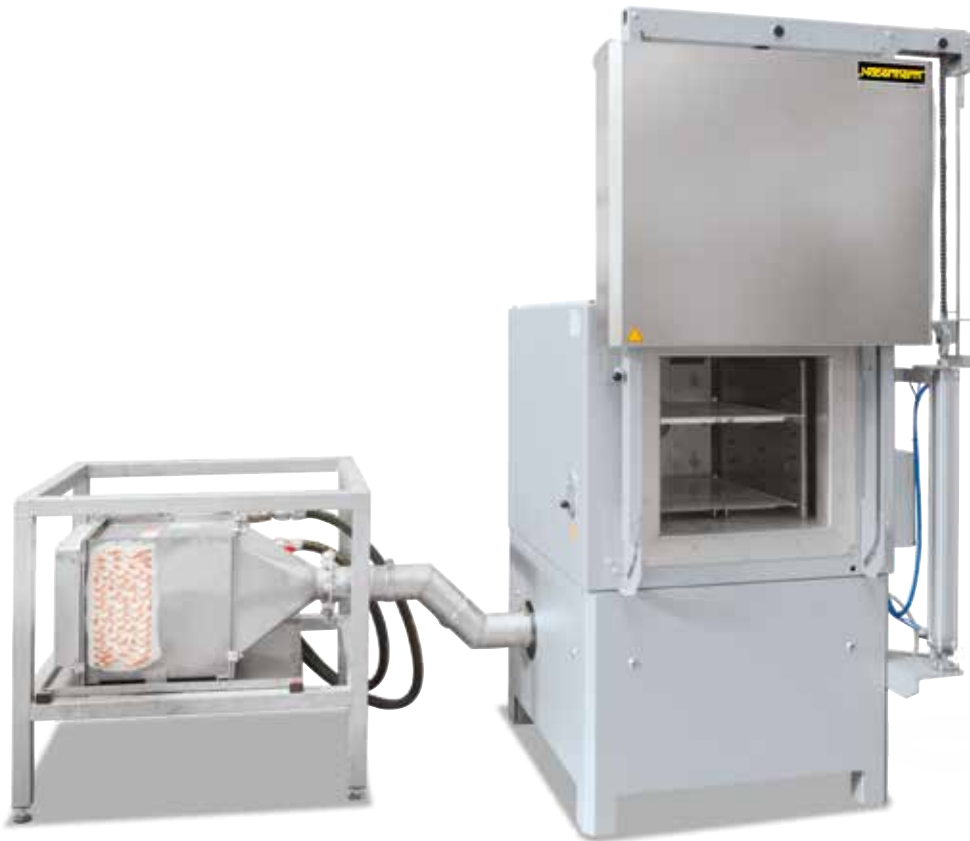
Forced convection chamber furnace NA 120/45 with fresh-air cooling
