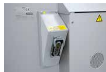
Plug socket on the furnace for the cable connection to the switchgear and control box
