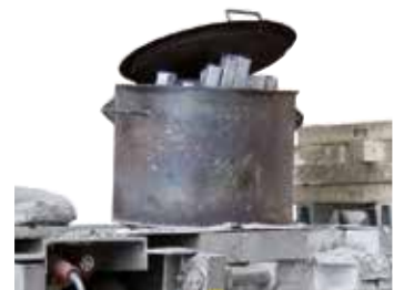
Charging funnel for ingots
