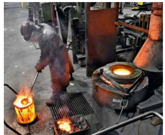
Bale-out furnace TB 20/14 in a pit with exhaust gas discharge over the crucible rime and swiveling collar plate for crucible pulling
