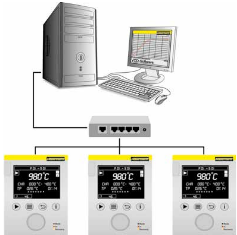
Example lay-out with 3 furnaces
