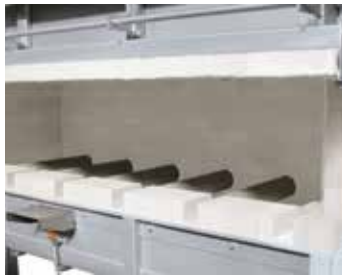
Indirect gas firing with radiation tubes
