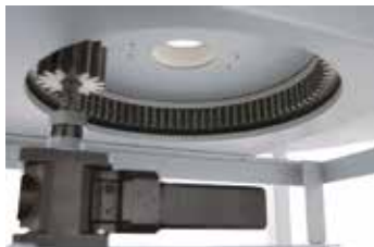
Gear rim drive under the rotary hearth furnace
