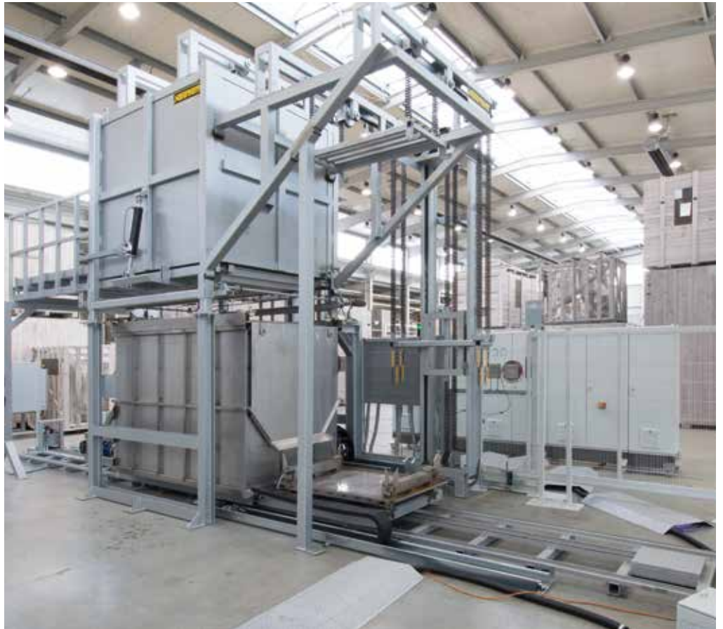
Fully automatic drop-bottom furnace with movable water bath, including holding position for charging and unloading crane
