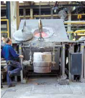
Charging of transport ladle with tilting furnace K 360/12
