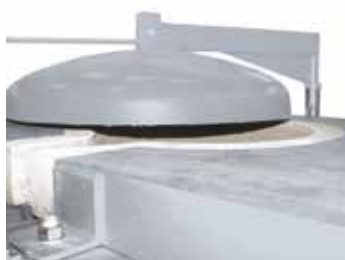
Swing lid with good sealing to collar plate to avoid heat loss over the crucible opening
