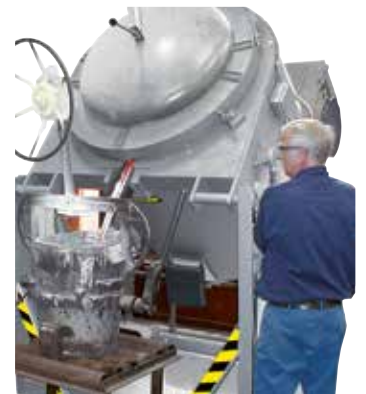
Tilting furnace KB 240/12 for melting aluminum alloys
