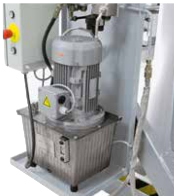
Hydraulic system with flame resistant hydraulic fluid
