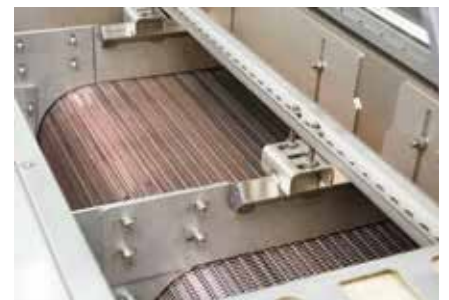
Mesh belt drive in continuous furnace D 1100/3600/100/50 AS
