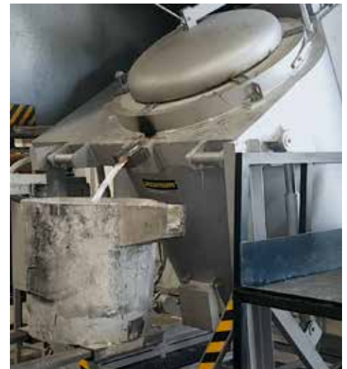
Tilting furnace KBR 240/11 during filling of a transport ladle
